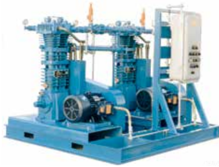
Duplex HD613 two-stage triple-seal compressors with control panel for natural gas pressure boosting operation.
