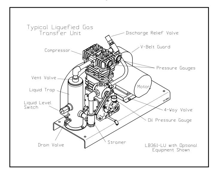
Blackmer 'LB' series compressors are specifically designed to transfer liquefied gasses like propane, butane and anhydrous ammonia. They are ideal for rail car unloading and vapor recovery applications. All models feature ductile iron pressure parts for greater resistance to both thermal and mechanical shock. Models are available for transfer rates of 35 to 700 gpm (132 to 2,630 lpm) to accommodate any size plant.
